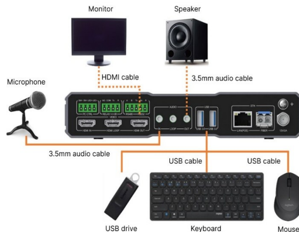
Fig 3-8 Decoder-KVM hardware connection
